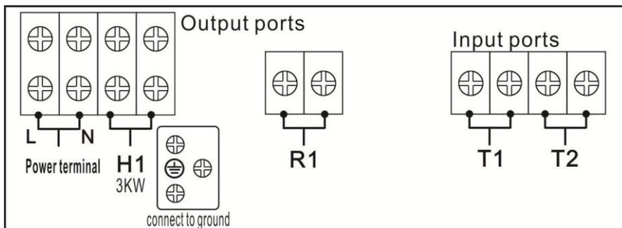
➤ **Power terminal N, L:** AC220V, 20A, for power connection, L: live wire, N: zero wire,
