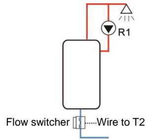
Tap seems like a remote controller, it controls the running of DHW pump. This control mode of DHW pump is an energy saving solution.
